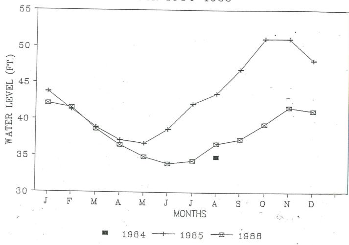
Figure 6 Average Monthly Groundwater Elevations Well A-20
