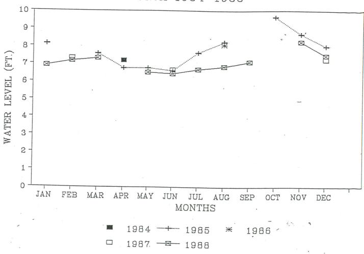
Figure 7 Average Monthly Groundwater Elevations Well EX-1
