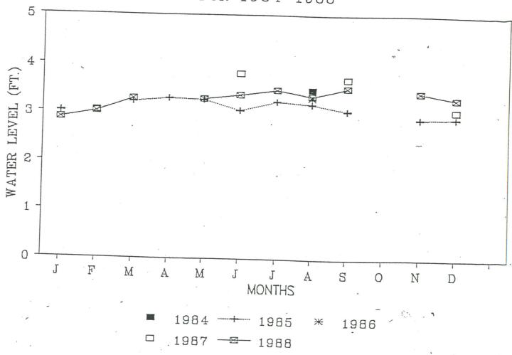
Figure 1 Average Monthly Groundwater Elevations Well EX-6
