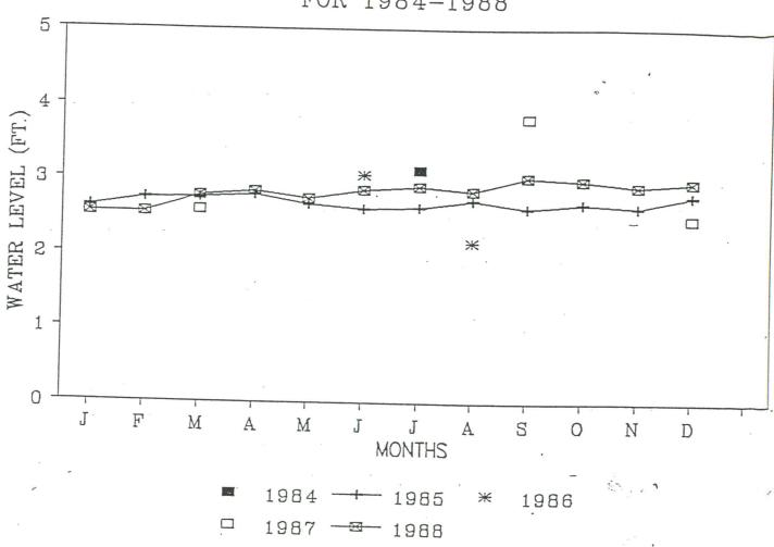
Figure 5 Average Monthly Groundwater Elevations Well EX-10
