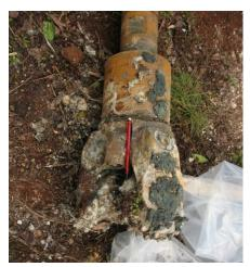
Figure 14. Evidence of contact with basement. Saprolitic material clinging to the drill bit, recovered from bottom of AECOM-3, which was drilled to the basement contact. Photograph taken 6 December 2010.
