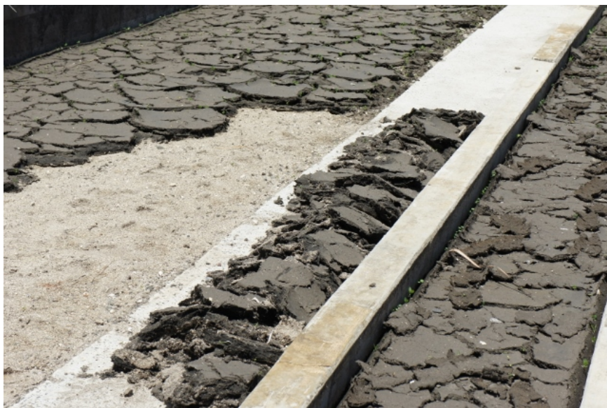
Figure 13. Air dried sludge with an estimated 50% moisture content. Image source: author.
