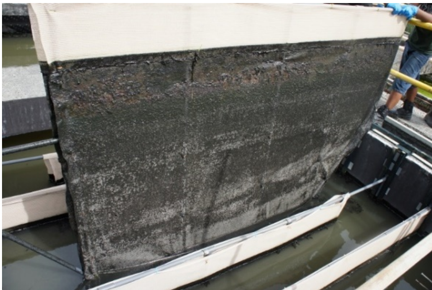
Figure 9. Inspection of a biocarrier sheet showing biofilm growth. Image source: author.
