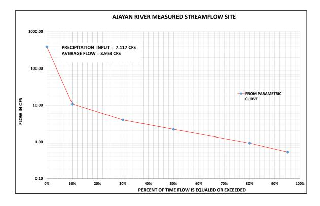
Figure 28. Flow duration curve for Ajayan River measured stream site
