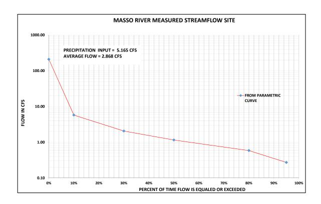
Figure 25 Flow duration curve for Masso River measured stream site
