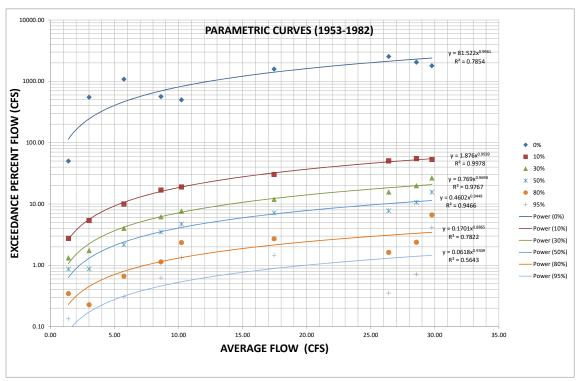
Figure 10. Parametric flow duration curves from 2014 study
