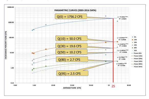
Figure 9. Use of parametric flow duration curves to predict flow duration values at an ungaged site with an average flow of 25 cfs (2016 Study)
