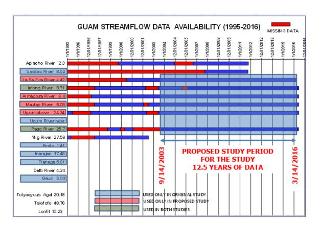
Figure 5. Availability of streamflow data from USGS gages on Guam
