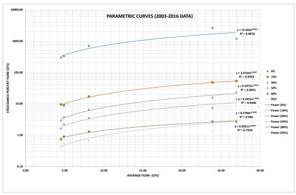
Figure 8. Parametric flow duration curves for South Guam streams
