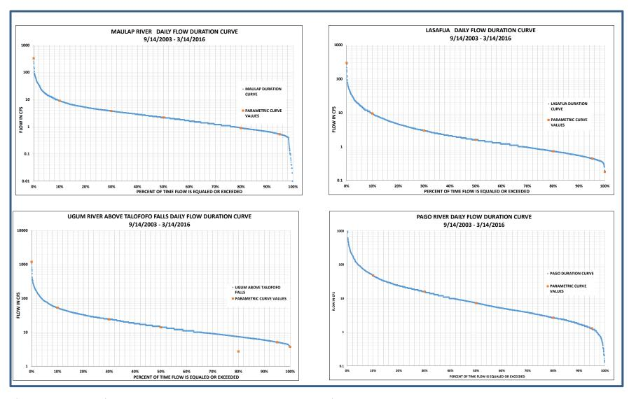
Figure 7. Flow duration curve for Maulap, Lasafua, Ugum, and Pago Rivers, Guam (2003-2016)
