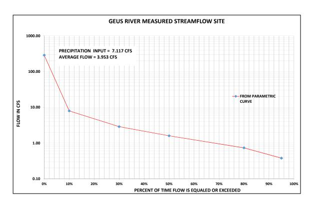
Figure 27 Flow duration curve for Geus River measured stream site
