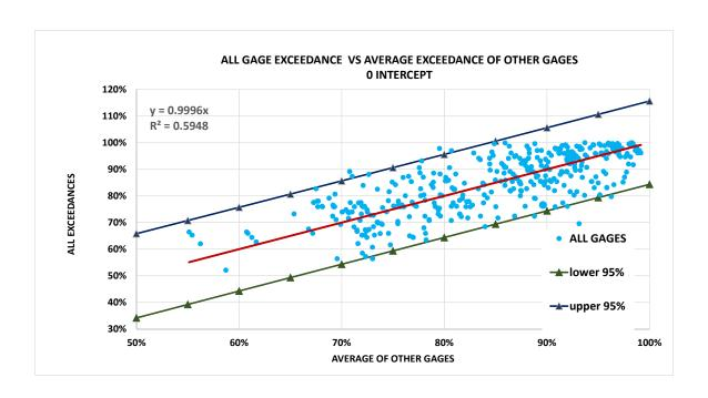
Figure 21. Confidence bounds for zero intercept regression analysis for all dummy gages combined
