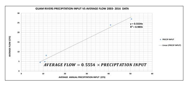
Figure 12. Average flow vs precipitation input for Guam's rivers (2016 data)
