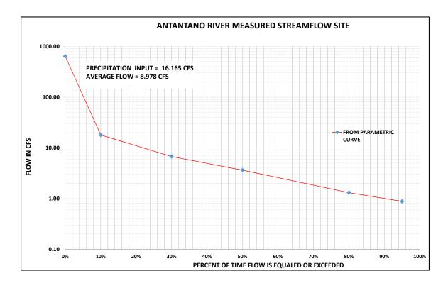
Figure 26. Flow duration curve for Atantano River measured stream site
