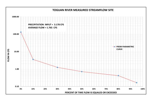
Figure 23 Flow duration curve for Toguan River measured stream site
