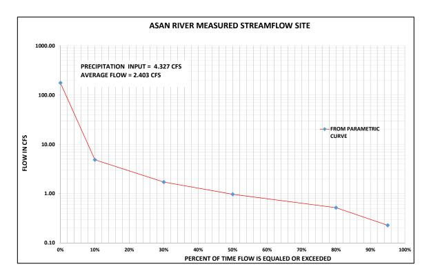
Figure 24. Flow duration curve for Asan River measured stream site
