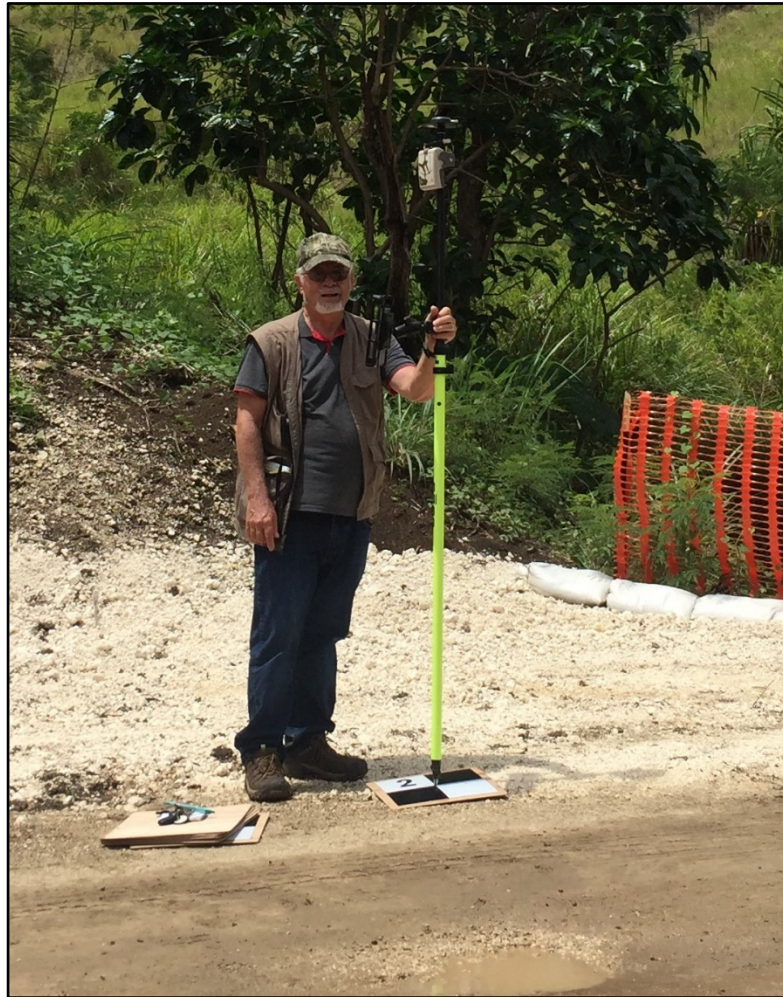
Figure35. A researcher gathering the location and elevation data for a GCP located along the Toguan River near Umatac, Guam using an EOS Arrow Gold GNSS rover receiver
