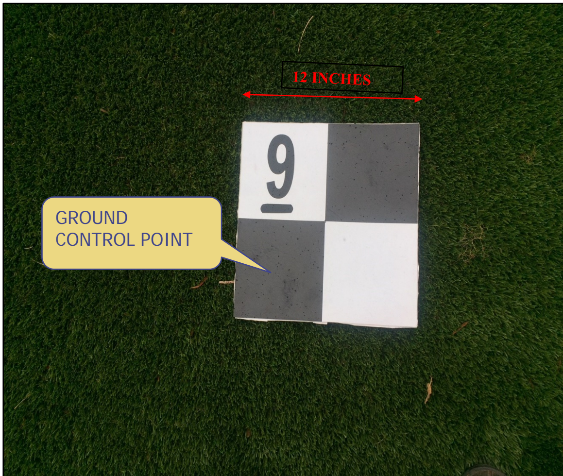
Figure 33. Sample Ground Control Point used for correcting orthographic and elevations models produced by processing applications
