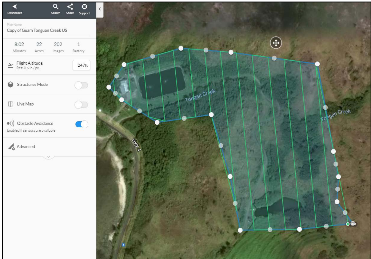
Figure 6. DroneDeploy application screen for planning a composite photo mission for the Toguan River near Umatac, Guam
