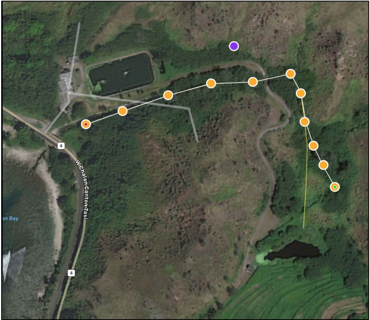
Figure 7. Maps Made Easy Drone Map screen for planning a single line photo mission for the Tongan River near Umatac, Guam
