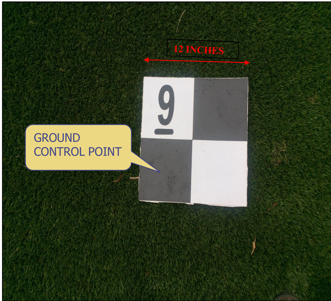
Figure 4. Sample Ground Control Point Used for Correcting Orthographic and DEMs Produced by the Processing Applications
