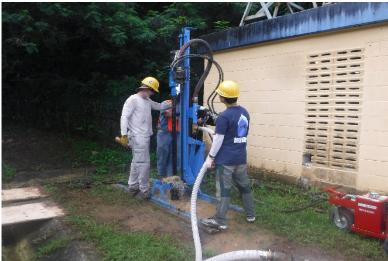
Figure 3.6. The Lonestar LH200 portable well drilling rig drilling hole 5 at the SRS.
