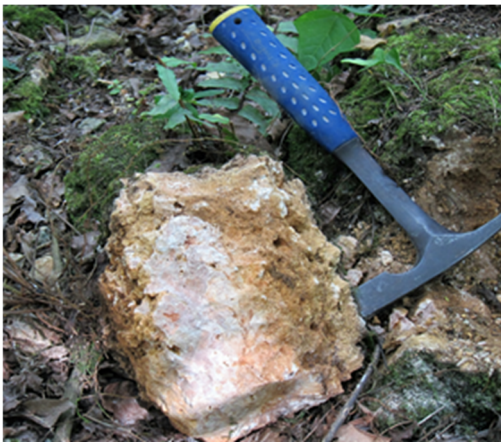
Figure 3.1. Sample of dense, hard, recrystallized Alifan Limestone collected at the old Navy quarry behind the SRS.
