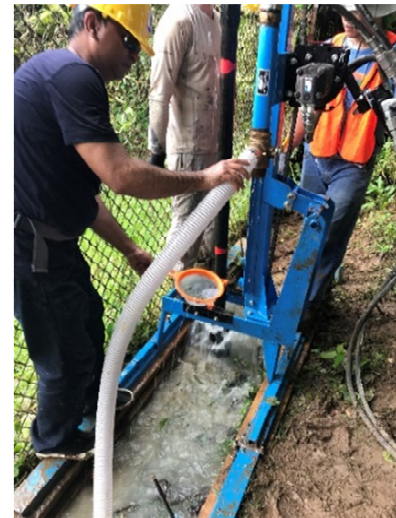
Figure 3.7. Collecting drilling samples with a sieve.
