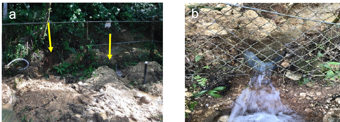
Figure 1.13. Overflow springs (a) Natural overflow conduits excavated outside of the southeastern fence, and (b) the V-notch weir installed to measure the flow rate.
