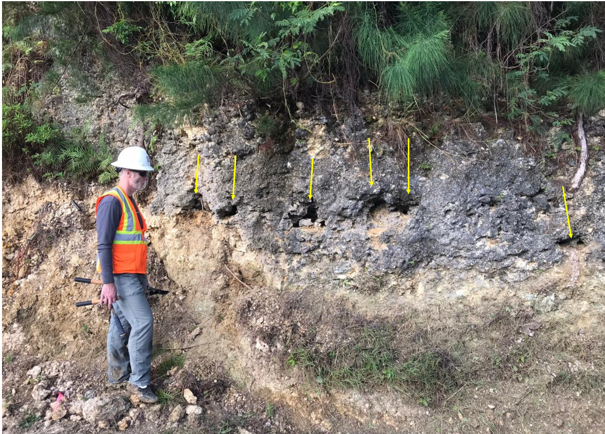
Figure 3.5 (c) Detail, showing distributed hand-scale cavernous porosity at the contact. The cut has intercepted and exposed the cross-section of a network of open conduits that have formed at the contact between the soluble, high-permeability limestone above and the insoluble, low-permeability clayey layer beneath. Although the ones seen here are inactive, conduits such as these drain the water from the overlying limestone aquifer and can be expected to be exposed at the SRS when the contact is excavated.
