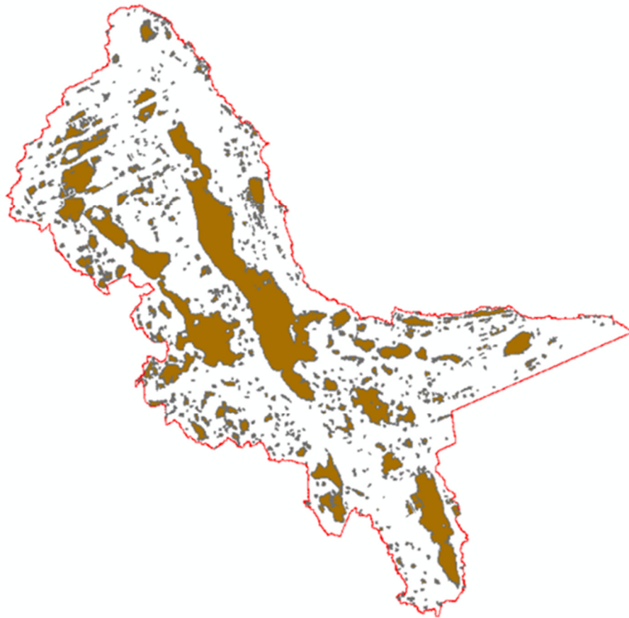
Figure 3.2. Fill area (area of closed surface depression).
