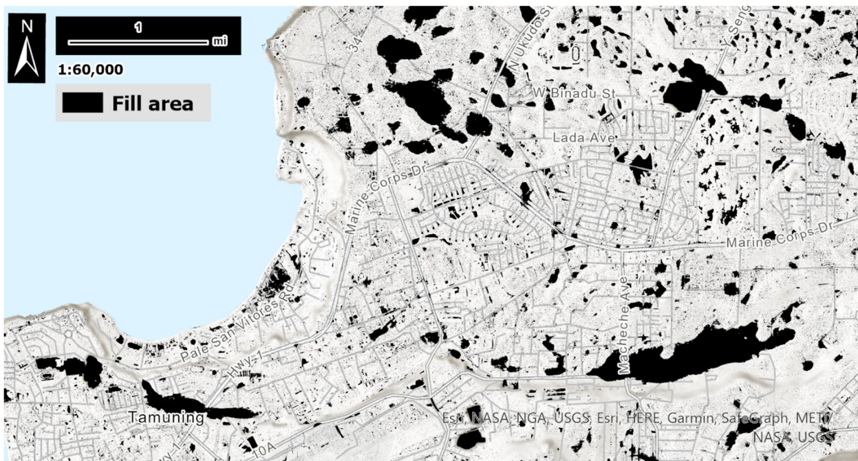
Figure 4.2 Fill area analysis feature, unfiltered. An undelimited fill analysis includes fill areas of less than 1 sqm that would produce an overwhelming delineation of insignificant watersheds. However, since sinkholes can be smaller than 1 sqm, a fill area or closed surface depression suggest that there may be a sinkhole within. Fill areas are often considered suspect sinkhole, as it may or may not have a sinkhole. Most surface depressions have a high probability of resulting in dolines in a karst terrain.
