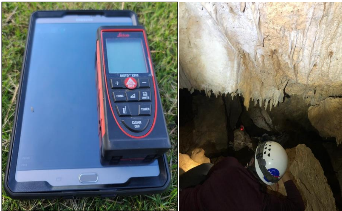
Figure 3.3. Digital cave survey tools (Disto-X and tablet) used to measure and map Ayuyu Cave.
