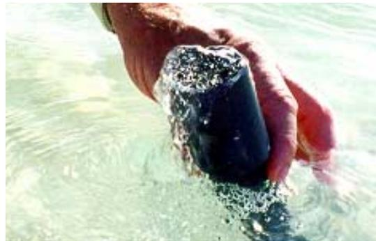
Figure 10. Fresh water flowing from PVC pipe pushed into the substrate in front of the Outrigger Hotel
